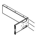
Use (3) M4 screws to secure ear bracket to panel.
